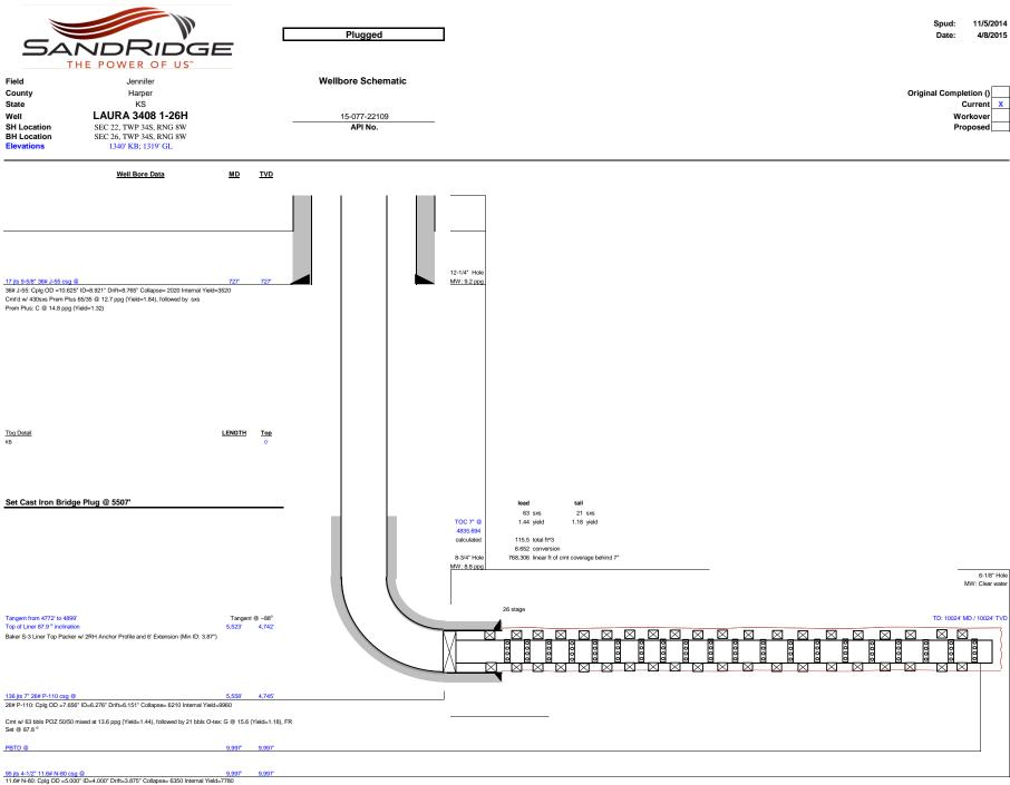
26 Stage Baker Fracpoint OH completion system ran, NO cement pumped.
