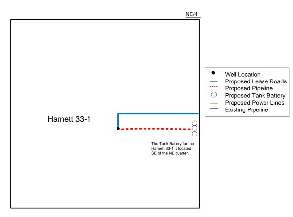
Proposed Details of NE/4 Sec 33 – T31S – R39W
