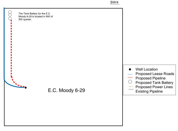
Proposed Details of SW/4 Sec 29 – T25S – R33W
