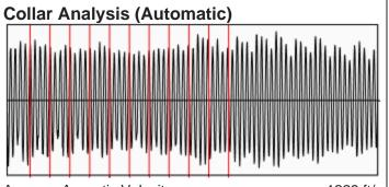
Average Acoustic Velocity Average Joints Per Sec. Joints To Liquid 1229 ft/s 19.39 Jts/sec 112.42 Jts
