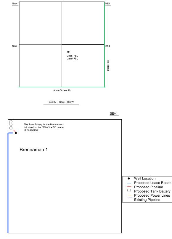
Proposed Details of SE/4 Sec 22 – T25S – R33W
