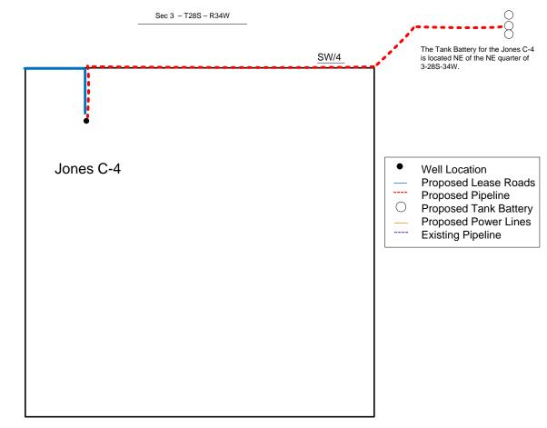
Proposed Details of SW/4 Sec 3 – T28S – R34W
