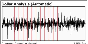
Average Acoustic Velocity Average Joints Per Sec. Joints To Liquid 1256 ft/s 19.32 Jts/sec 137.32 Jts
