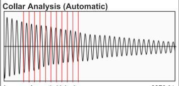
Average Acoustic Velocity Average Joints Per Sec. Joints To Liquid 2279 ft/s 35.06 Jts/sec 411.97 Jts
