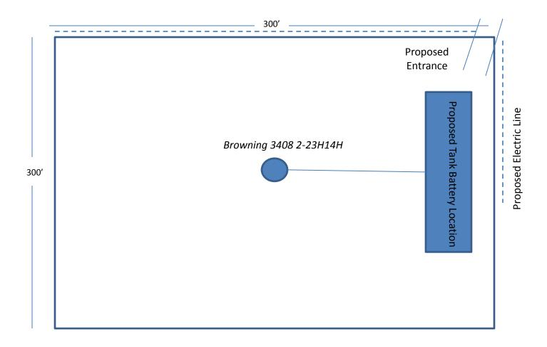
This plat is for proposed information only and may not represent the final drilling pad layout of wells, utilities or tank battery. Conservation Division 266 N. Main St., Ste. 220 Wichita, KS 67202-1513
