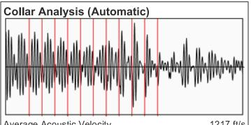
Average Acoustic Velocity Average Joints Per Sec. Joints To Liquid 1217 ft/s 18.72 Jts/sec 40.22 Jts
