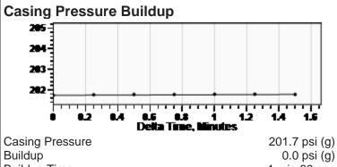
**Buildup Time** 1 min 30 sec Gas Gravity 0.7526 Air = 1
