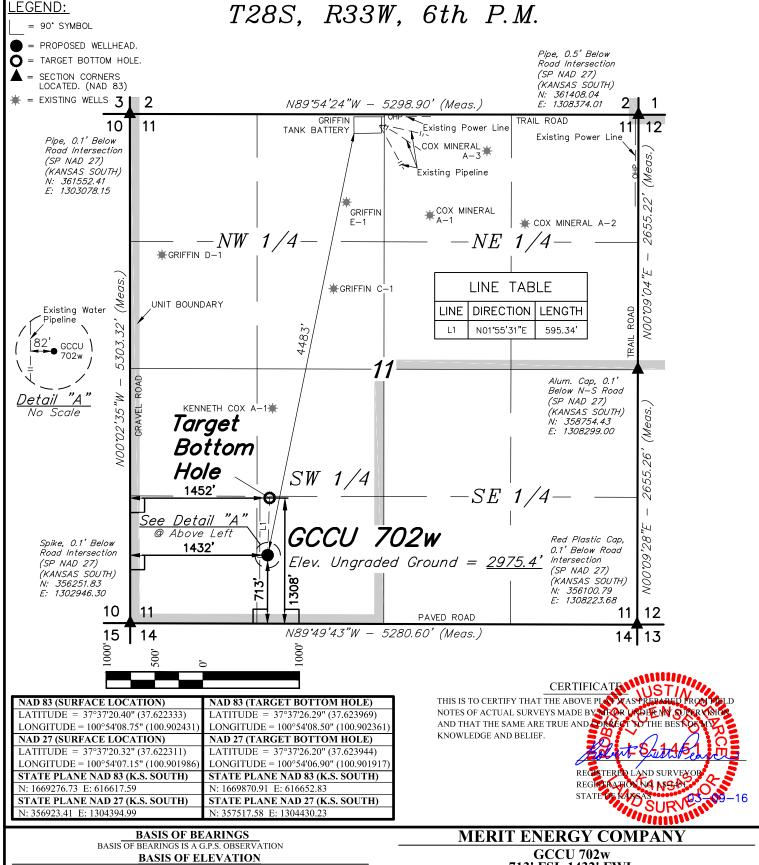
THE BASIS OF ELEVATION, ELEV: 2943.84' WAS DERIVED FROM AN OPUS SOLUTION AT LAT: 37°33'17.64" LONG: 100°53'21.35" AND HAS A DATUM OF NAVD88.
