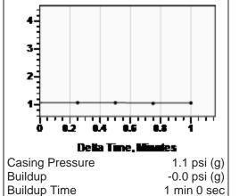
Casing Pressure Buildup
