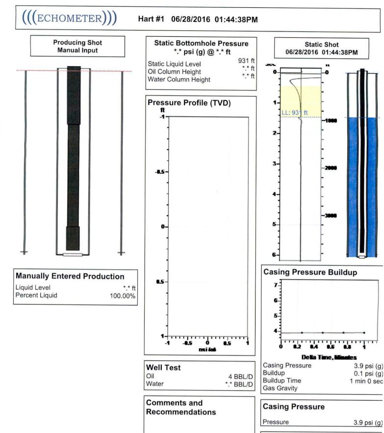
Static test taken for TA well.
