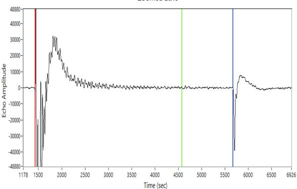
Depth: 1795.50 ft Return Time: 4.25 sec Acoustic Velocity: 845.34 ft/s Average Joint Length: 31.50 ft
