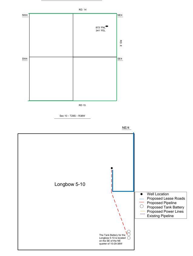
Proposed Details of NE/4 Sec 10 – T29S – R38W
