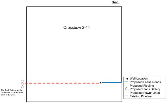
Proposed Details of NW/4 Sec 11 – T29S – R38W
