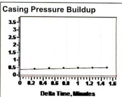
Casing Pressure Buildup Buildup Time Gas Gravity 0.4 psi (g) 0.2 psi (g) 1 min 30 sec
