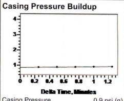
Casing Pressure Buildup Buildup Time Gas Gravity 0.9 psi (g) 0.1 psi (g) 1 min 15 sec
