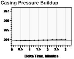
Casing Pressure Buildup Buildup Time Gas Gravity 263.9 psi (g) 0.1 psi (g) 3 min 0 sec
