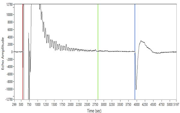
Depth: 2047.50 ft Return Time: 3.40 sec Acoustic Velocity: 1205.12 ft/s Average Joint Length: 31.50 ft Number of Joints: 65.00
