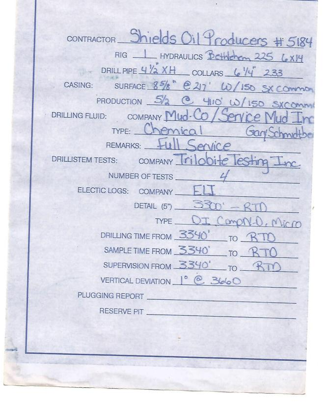
**DAILY REPORT** DATE: 7 a.m. Depth **RIG ACTIVITY** 5-25-17 MIRU S.PUD 5.30.17 220' 5.31.17 W. O.C. 6-01-17 1209' Orilling Sh. Slitst 2270' 6.02.17 Irilling sh sitst + 3002 6.03.17 rilling sh stat P 6.04-17 3472' rilling Top-Ka LKC. A+ 6.05.17 3ldo) ST -#1 DST # 2 LKC.C.F 3725 6.00.17 Dillus Base KC 6.07.17 3872' STHY Arbuckle 4/10' -T.D. 6-08-17
