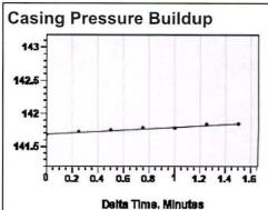
Casing Pressure Buildup Buildup Time 141.7 psi (g) 0.2 psi (g) 1 min 30 sec
