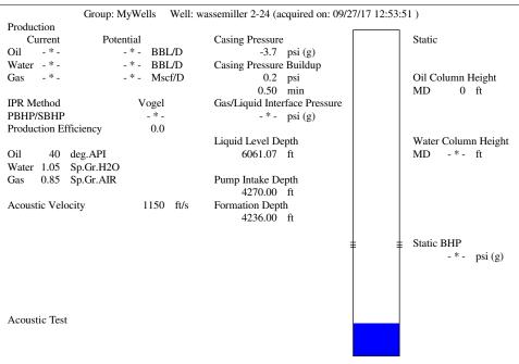
Entered Acoustic Velocity for Liquid Level depth determination
