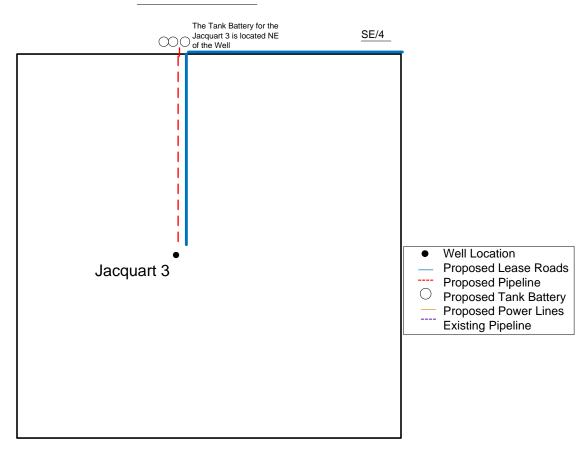
Proposed Details of SE/4 Sec 15 – T28S – R34W
