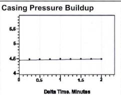
Casing Pressure Buildup Buildup Time Gas Gravity 4.4 psi (g) 0.0 psi (g) 2 min 0 sec
