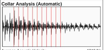
Average Acoustic Velocity Average Joints Per Sec. Joints To Liquid 1316 ft/s 21.29 Jts/sec 124.66 Jts
