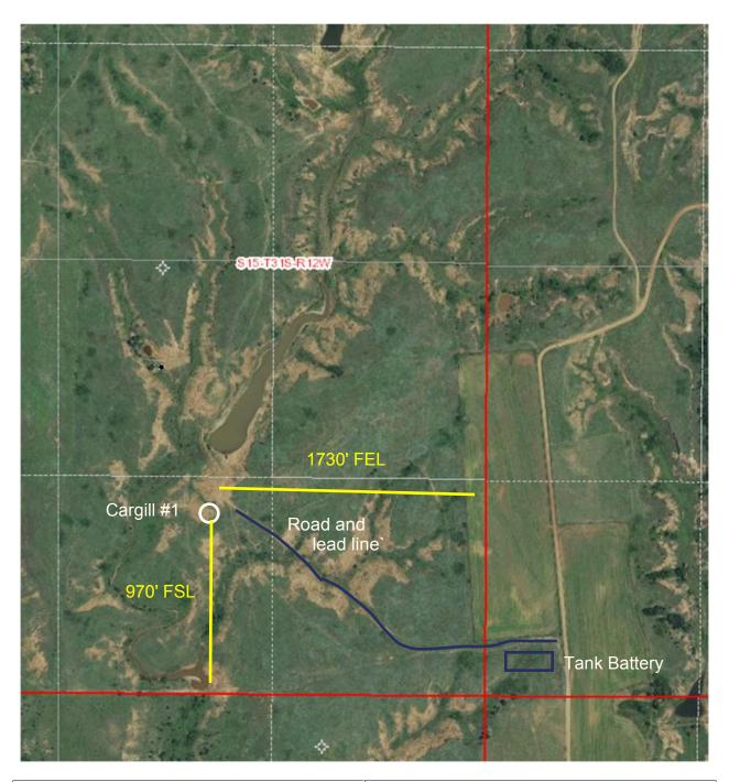
WHITE EXPLORATION, INC. CARGILL #1 970' FSL and 1730' FEL Section 15-31S-12W Barber County, Kansas Kansas Surface Owner Notification Act NON-BINDING ESTIMATE Of location of well, tank battery, road, etc
