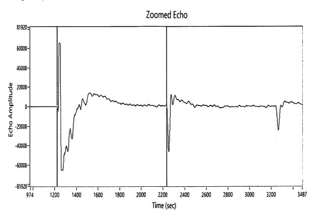
723.35 ft Depth: Return Time: 1.01 sec Acoustic Velocity: 1428.13 ft/s Average Joint Length: 31.45 ft Number of Joints: 23.00
