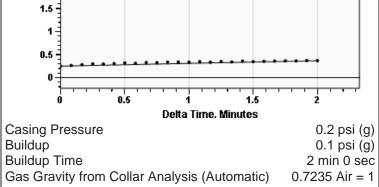
Casing Pressure Buildup
