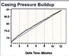
Casing Pressure Buildup Buildup Time Gas Gravity 78.7 psi (g) 2.2 psi (g) 12 min 0 sec
