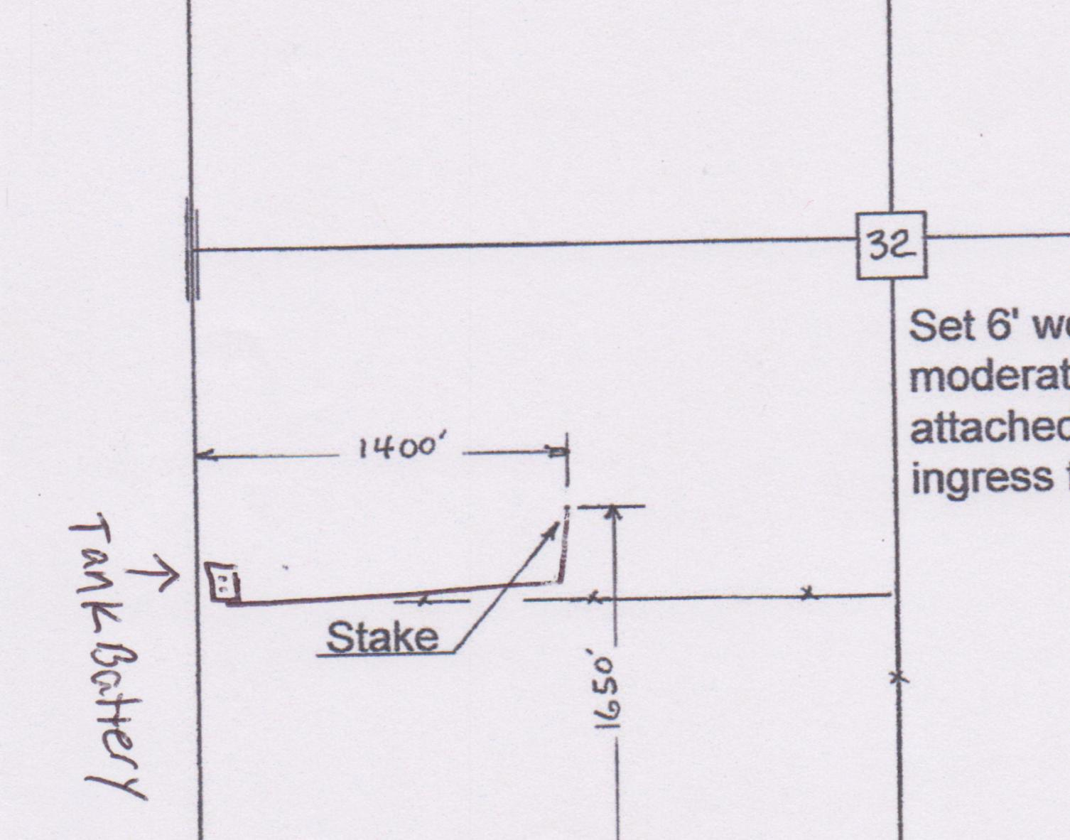
Set 6' wood stake on slight to moderate slope wheat. See attached for staking ingress. No ingress flagged.
