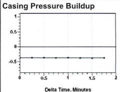
Casing Pressure Buildup Buildup Time -0.4 psi (g) -0.0 psi (g) 1 min 45 sec
