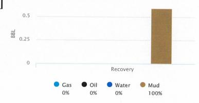
Initial Hydrostatic Pressure 2301 **PSI** Initial Flow 55 to 56 **PSI Initial Closed in Pressure** 1057 **PSI** Final Flow Pressure 62 to 66 PSI **Final Closed in Pressure** 1006 **PSI** Final Hydrostatic Pressure 2284 **PSI** Temperature 111 °F Pressure Change Initial 4.8 %
