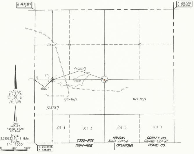
Distances shown in (parenthesis) are calculated based upon the Quarter Section being 2640 feet, those shown in [brackets] are based on GLO (General Land Office) distances and have <u>NOI</u> been measured on the ground.
