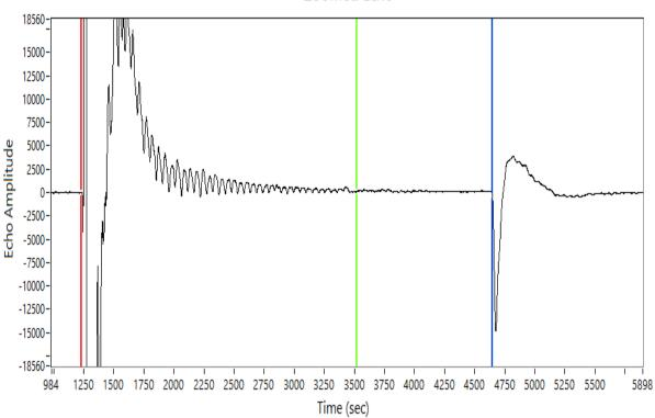
Depth: 2079.00 ft Return Time: 3.41 sec Acoustic Velocity: 1217.93 ft/s Average Joint Length: 31.50 ft Number of Joints: 66.00
