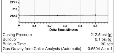
Casing Pressure Buildup
