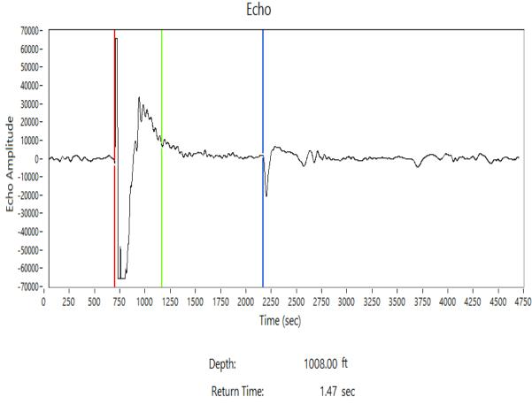
Acoustic Velocity: 1373.30 ft/s Average Joint Length: 31.50 ft Number of Joints: 32.00
