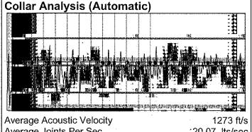
Average Joints Per Sec. '20.07 Jts/sec Joints To Liquid 138.93 Jts
