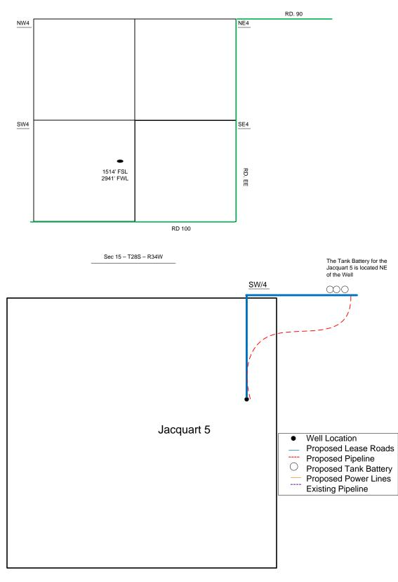
Proposed Details of SW/4 Sec 15 – T28S – R34W
