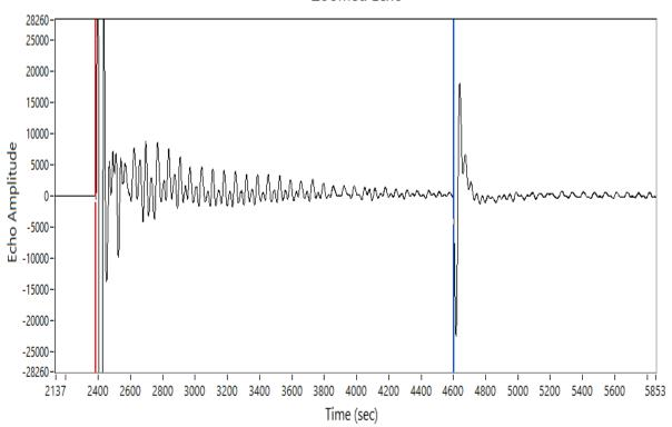
Depth: 990.00 ft Return Time: 2.22 sec Acoustic Velocity: 893.50 ft/s Average Joint Length: 30.00 ft Number of Joints: 33.00
