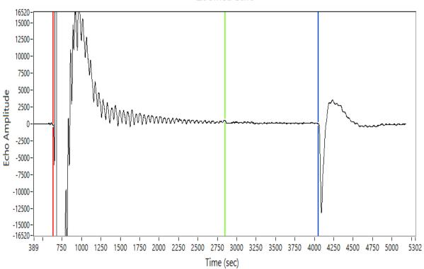
Depth: 2079.00 ft Return Time: 3.41 sec Acoustic Velocity: 1218.28 ft/s Average Joint Length: 31.50 ft Number of Joints: 66.00
