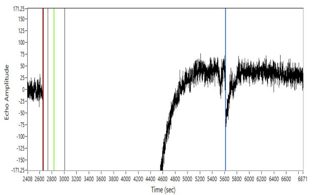
1080.00 ft Depth: Return Time: 2.96 sec Acoustic Velocity: 728.99 ft/s Average Joint Length: 30.00 ft Number of Joints: 36.00
