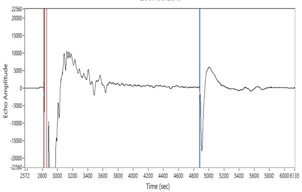
Depth: 1147.00 ft Return Time: 2.06 sec Acoustic Velocity: 1111.97 ft/s Average Joint Length: 31.00 ft Number of Joints: 37.00
