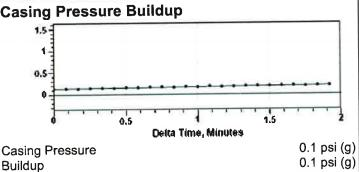
Casing Pressure Buildup 1 min 55 sec Buildup Time 0.7080 Air = 1Gas Gravity from Collar Analysis (Automatic)
