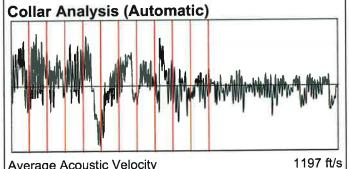
Average Acoustic Velocity Average Joints Per Sec. Joints To Liquid 1197 ft/s 18.88 Jts/sec 110.57 Jts
