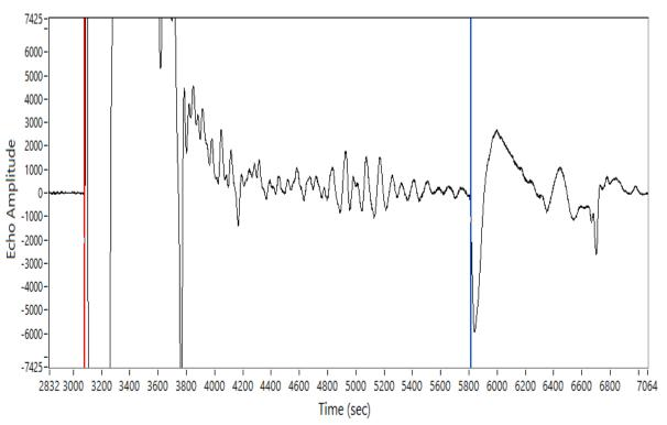
1008.00 ft Depth: Return Time: 2.73 sec Acoustic Velocity: 737.92 ft/s Average Joint Length: 31.50 ft Number of Joints: 32.00
