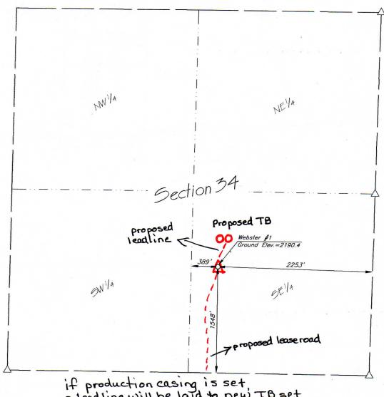
if production casing is set a lead line will be laid to new TB set
