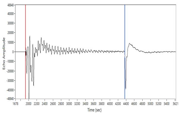
1121.76 ft Depth: Return Time: 2.44 sec Acoustic Velocity: 918.35 ft/s Average Joint Length: 31.16 ft Number of Joints: 36.00
