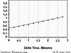
$\begin{array}{lll} \text{Casing Pressure} & 0.5 \text{ psi (g)} \\ \text{Buildup} & 0.6 \text{ psi (g)} \\ \text{Buildup Time} & 2 \text{ min } 45 \text{ sec} \\ \text{Gas Gravity} & 0.8497 \text{ Air} = 1 \\ \end{array}$
